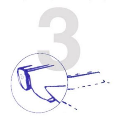
Put the mechanism with your right hand and take out the key pin from the hole. Now the mechanism is active.
